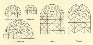
FIG. 149—PLANS OF THE EAST ENDS OF FIVE GOTHIC CHURCHES, ILLUSTRATING THE DEVELOPMENT OF THE CHEVET
