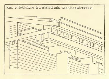
FIG. 22—IONIC ENTABLATURE, RETRANSLATED INTO WOOD. (AFTER DURM)
