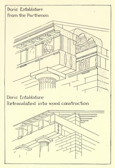
FIG. 20—THE GREET DORIC ORDER, WITH A RETRANSLATION INTO WOOD, (AFTER DURM)
