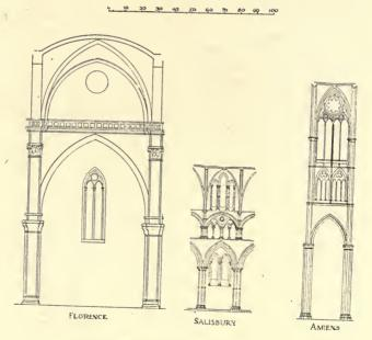
FIG. 140—SECTIONS AND SYSTEMS OF GOTHIC BUILDINGS
