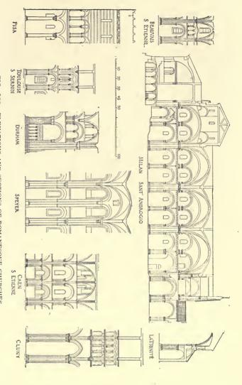
FIG. 100-ELEVATIONS AND SECTIONS OF ROMANESQUE CHURCHES
