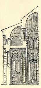
FIG. 120—CLERMONT - FER-RAND. NOTRE DAME DU PORT, TRANSVERSE SECTION, SHOW-ING HALF - BARREL VAULT OVER THE AISLE
